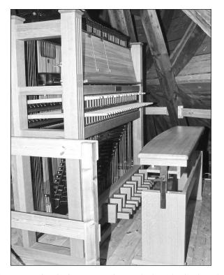
The automatic playing system is attached to the keyboard and uses the clappers to strike the bells by depressing the keys. The clappers are screwed into their fastenings inside the bell allowing them to be vertically adjusted to hit the best strike spot and are connected to the keyboard by wires attached to directed cranks. The medium-sized and small bells have a round piece of bronze instead of a crown attached to the top of them to isolate them from the bell frame.
