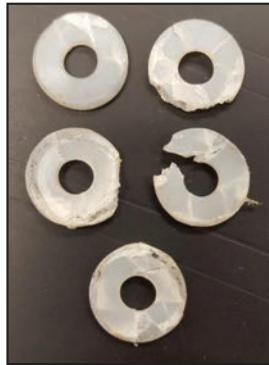
Affected plastic adjuster spacers from a carillon console
