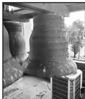
Three large major third bells, showing their distinctive bulge around the middle
