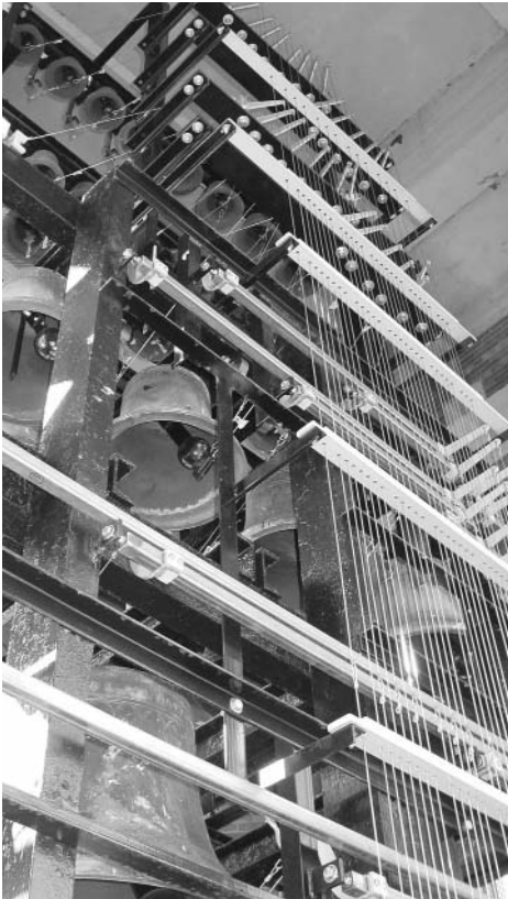
New transmission: looking up past the third level to radial action for trebles
