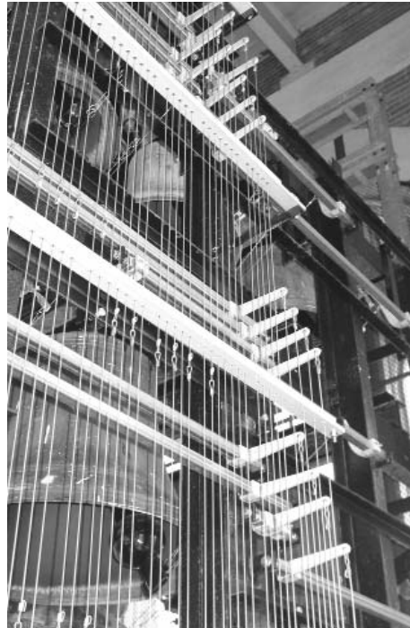
New transmission: tumbler action for basses and mediums
