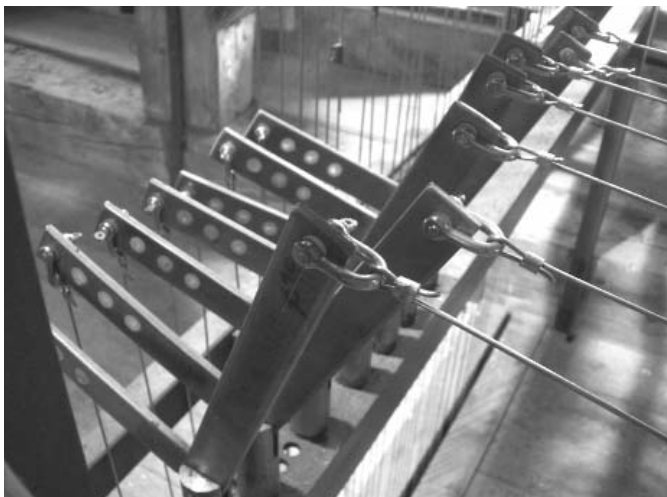
This is the best picture of the worst situation: the crank is in reverse position! The vertical wire at the horizontal crank arm (left) goes down to the keyboard and needs no holes for adjusting. The horizontal wire on the vertical crank arm (right) goes to the clapper. This arm needs holes in order to be able to adjust the sound of the bell. The person who installed this didn't know what he/she was doing! One small "positive" fact in this disastrous picture: the builder uses shackles for connecting wires.
