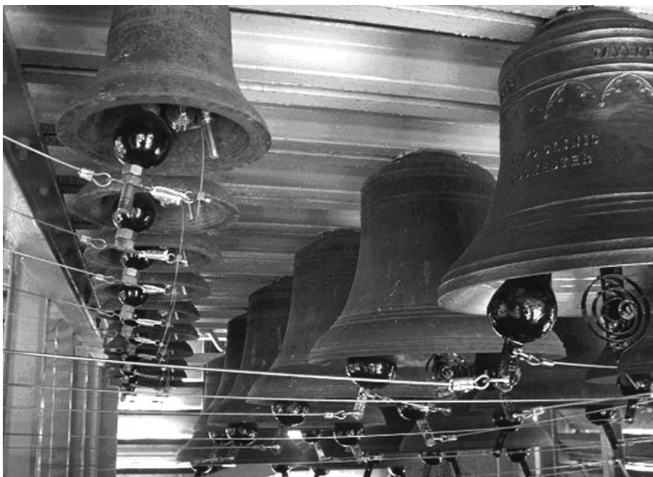
New clapper assemblies and spring mounts for Petit & Fritsen bells (left row), restored Gillett & Johnson clappers and springs (center foreground), and the new Taylor bell (right).
