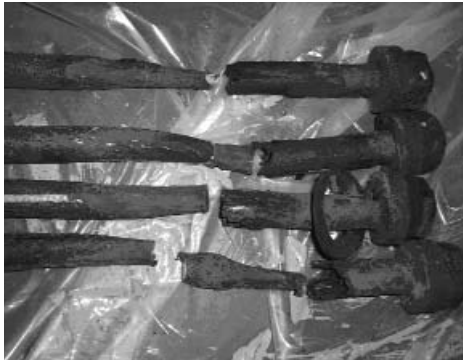
Photo showing the extensive deterioration of the suspension bolts (bourdon).
